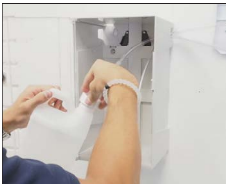
Screw Rite-Connect caps onto chemical bottles. (New bottles will have Rite-Connect single flow inserts in them.)
