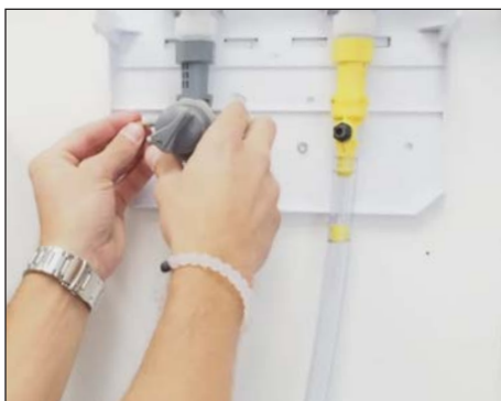
Choose metering tip(s) based on Essential Tip Guide and insert into necessary discharge ports at dispenser.
