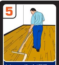
Apply two coats of Sport Seal (226SF). Allow it to dry for 12 hours under normal conditions - longer under humid conditions.
