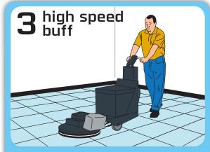
Buff the entire facility using a high speed machine and buffing pads. Turn pads often to prevent pad loading. Always dust mop after buffing.
