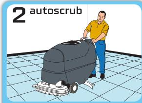
Autoscrub the floor with red pads and a  $\frac{1}{2}$  oz./gal. dilution of Blue Concentrate #56 from the Emax dispenser. Pick up the trail left by the autoscrubber with a mop and bucket of clean, cold water. For hard-to-reach areas and for facilities not equipped with a scrubber, all floors must be damp mopped. Use a clean mop and a  $\frac{1}{2}$  oz./gal. solution of Blue Concentrate #56 Allow floors to dry before buffing.
