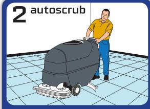
Autoscrub the floor with red pads and a 6 oz./gal. dilution of Citrus Scrub 'N Shine #12. Pick up the trail left by the autoscrubber with a mop and bucket of clean, cold water. For facilities not equipped with a scrubber, all floors must be damp mopped. Use a clean mop and 6 oz./gal. solution of Citrus Scrub 'N Shine #12. Allow floors to dry before buffing.
