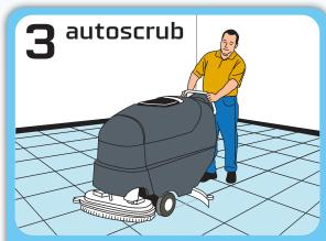
Autoscrub the floor with red pads and a 2 oz./gal.\* dilution of Neutral Cleaner. Pick up the trail left by the autoscrubber with a mop and bucket of clean, cold water.
