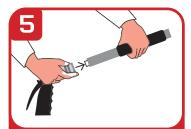
Remove foam wand from spray gun by pulling back the quick connect. Return foam wand to storage hook.
