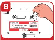
Turn Rinse lever to OFF (horizontal) position and move Sanitizer lever to ON (up) position.
