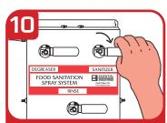
When finished, return all levers to the OFF (horizontal) position.
