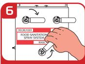
Turn Degreaser lever to OFF (horizontal) position and move Rinse lever to ON (up) position.
